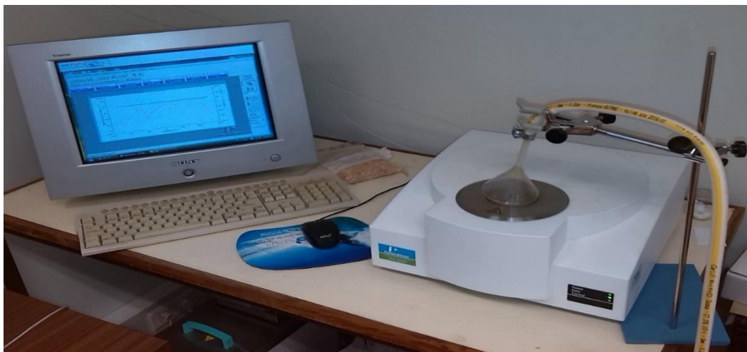
Figure 10. TG/DSC STA 6000 Simultaneous Thermal Analyzer
